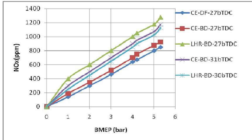
**Figure 5: Variation of Nitrogen Oxide Levels with Brake Mean Effective Pressure (BMEP) in Conventional Engine (CE) and Engine with LHR Combustion Chamber at Recommended Injection Timing and Optimum Injection Timing and at an Injector Opening Pressure of 190 Bar With Biodiesel (BD)**
