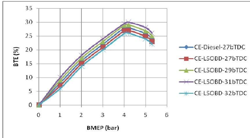
**Figure 2: Variation of Brake Thermal Efficiency (BTE) with Brake Mean Effective Pressure (BMEP) in Conventional Engine (CE) and with Various Injection Timings at an Injector Opening Pressure of 190 Bar with Biodiesel**
