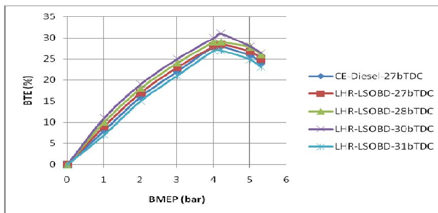
**Figure 3: Variation of Brake Thermal Efficiency (BTE) With Brake Mean Effective Pressure (BMEP) in LHR Combustion Chamber at Different Injection Timings with Biodiesel (LSOBD) Operation**
